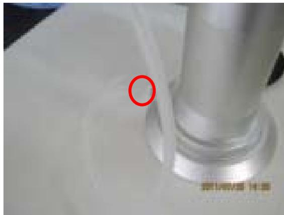
**Please plug the blowing pipe to machine and arm head in turn.**
