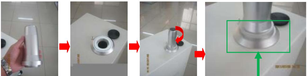
Please install the port of laser output, and tighten as the arrow showing.
